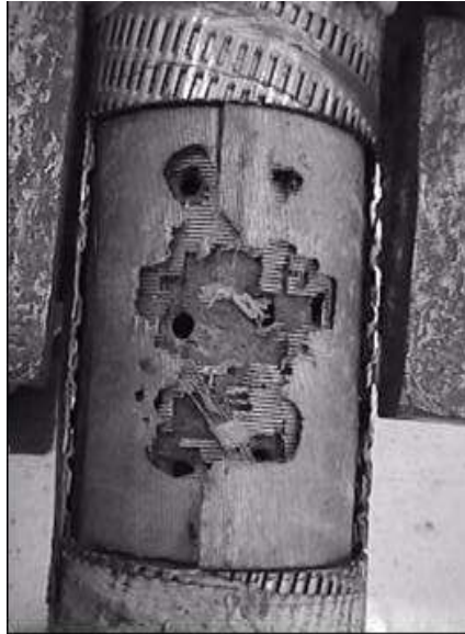
Eroded sand screen
