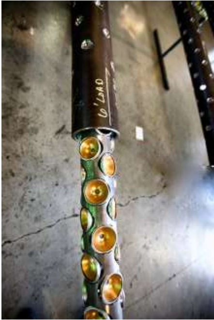
TCP Gun Carrier and charges (Courtesy of The Expro Group)
