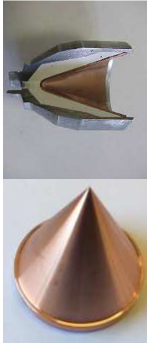
Charge and Shaped liner (Courtesy of Springer)
