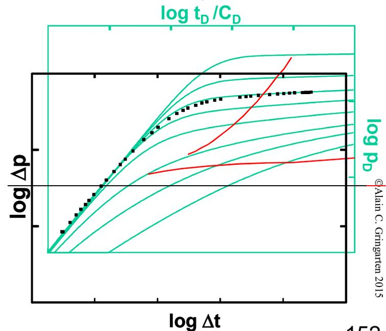
**STEP 2: Final Type Curve Match for a Well with Wellbore Storage and Skin in a Reservoir of Infinite Extent with Homogeneous Behaviour**
