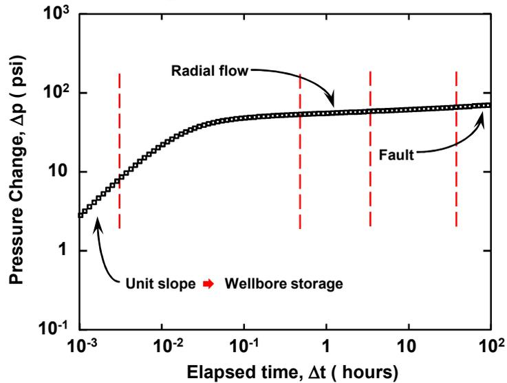
high conductivity fracture in a reservoir with homogeneous behaviour and a fault
